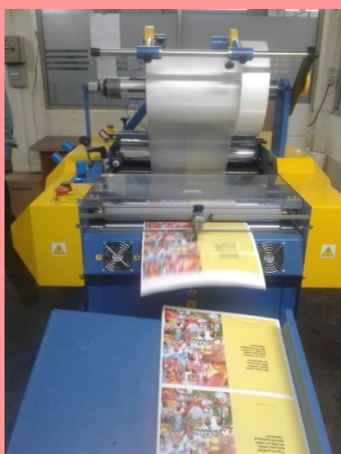
Laminating Machine Machine which is Laminating book covers.
