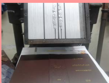
This Machine Printed State Logo, books name and details of silver and gold on the reekshin covers are printing in shiny color.
