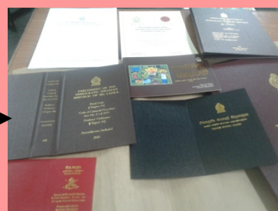
This Machine Printed State Logo, books name and details of silver and gold on the reekshin covers are printing in shiny color.
