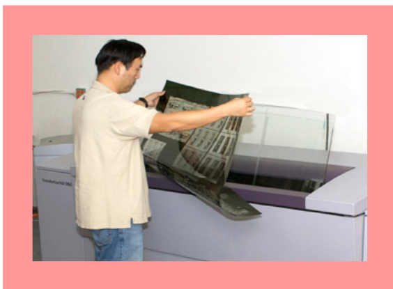
Image Setter Machine - Inserting Film to make Plate and Blocks.
