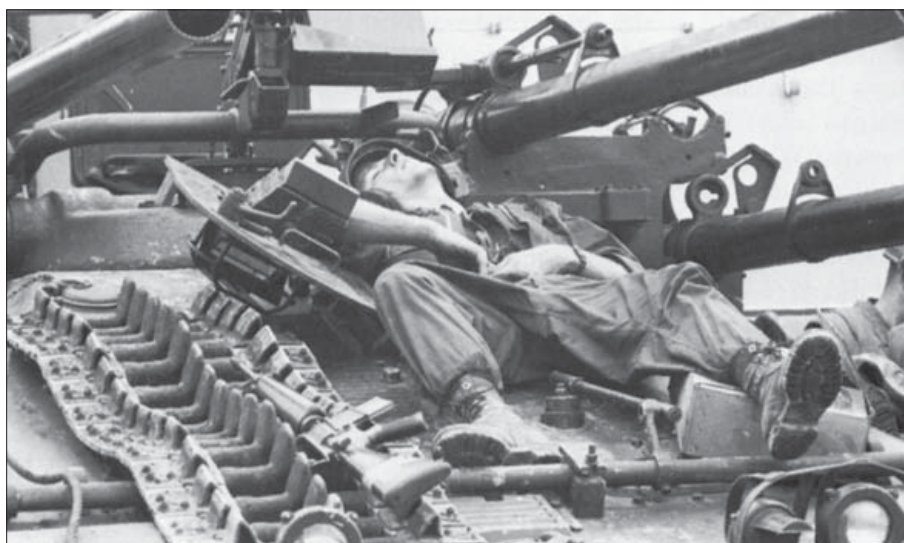
A Marine Ontos crewman lays exhausted across the front of his vehicle. The 106mm recoilless rifle, six of which were mounted on the Ontos' lightly armored frame, was the perfect weapon for punching holes in the sides of Hue's concrete buildings. The dust cloud raised by firing the weapon also provided concealment as the Marines rushed across streets to assault buildings. (NARA)
