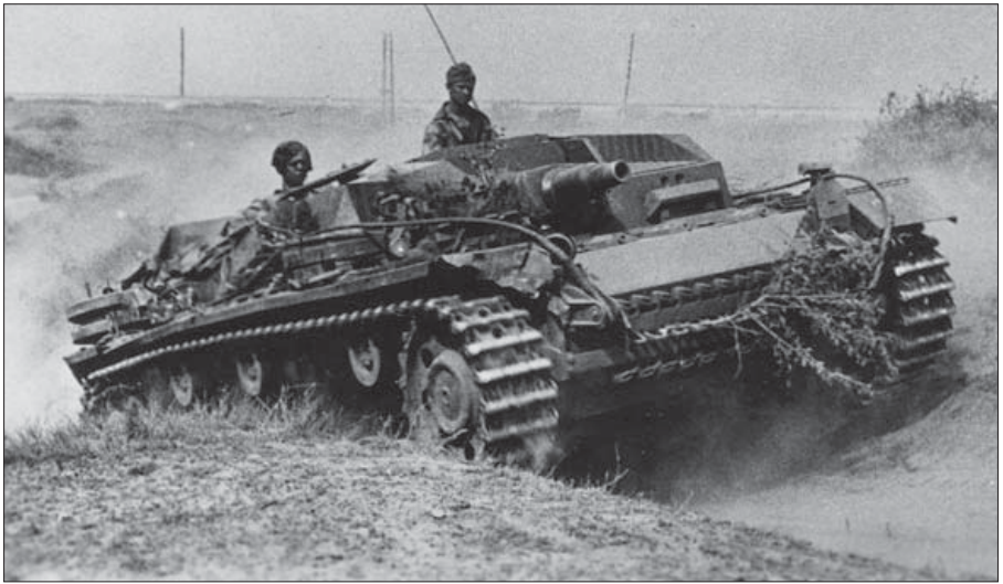
A Sturmgeschütz IIIa (StuG IIIa) maneuvers through the dust of Stalingrad in September 1942. The Sturmgeschütz III was a tracked infantry support vehicle, not a tank, and specifically designed to assist infantry reduce fortifications. It did not have a turret but had very thick frontal armor and was ideal for urban warfare. (Bundesarchiv)
